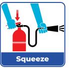
Squeeze the operating lever to discharge the fire extinguishing agent.
