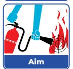
Aim the nozzle or hose at the base of the fire from the recommended safe distance.
