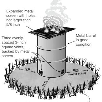
Ground cleared down to mineral soil or gravel at least 10 feet on each side of incinerator
