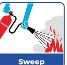
Starting at the recommended distance. sweep the nozzle or hose from side to side until the fire is out. Move forward or around the area as the fire diminishes. Watch the area in case of re-ignition.
