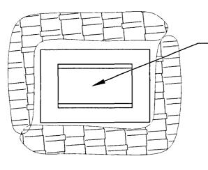
INSTALL FILTER FABRIC UNDER INLET GRATE IMMEDIATELY UPON INSTALLATION. REMOVE AND REPLACE WITH NEW FABRIC REGULARLY TO MAINTAIN FLOW AND REDUCE SEDIMENT ACCUMULATION.
