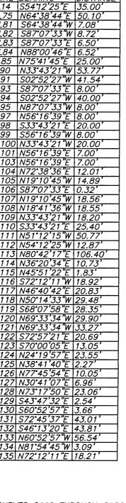
NOTE: LINES L112 THROUGH L135 AND CURVES C119 THROUGH C126 ARE SHOWN TO TIE THE WETLANDS BUFFER TO PHASE 3 BOUNDARY LINES.
