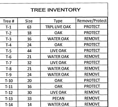
TREE TABLE NOTES: PROTECT: INDICATES TREE CONSIDERED PROTECTED BY THE LDC AND IS PROPOSED TO REMAIN ONSITE UPON DEVELOPMENT. CONTRACTOR SHALL INSTALL TREE BARRICADES PER TREE BARRICADE DETAIL IN THIS PLAN
